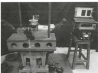
Fig.3 Calibration experiment platform of six-dimensional force sensor 图 3 六维力传感器标定实验台
