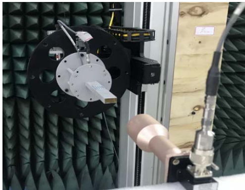
Fig.7 Measurement setup of dual-mode conical horn antenna 图 7 双模圆锥喇叭天线测量
