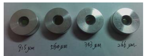
Fig.2 Test samples of effective second-order nonlinear coefficient of DAST crystals 图 2 DAST 晶体有效二阶非线性系数测试样品
