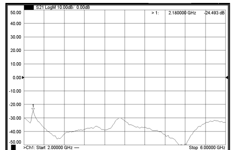
Fig.6 Measured isolation from the port 1 to port 2 图 6 端口 1 和 2 隔离度测试曲线
