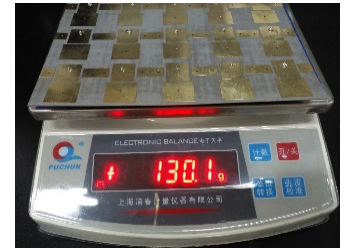
Fig.7 The weight test of antenna sample 图7 天线样品质量测试
