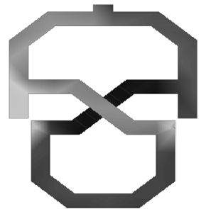
Fig.6 Model of the oscillator inductance 图 6 振荡器电感模型图
