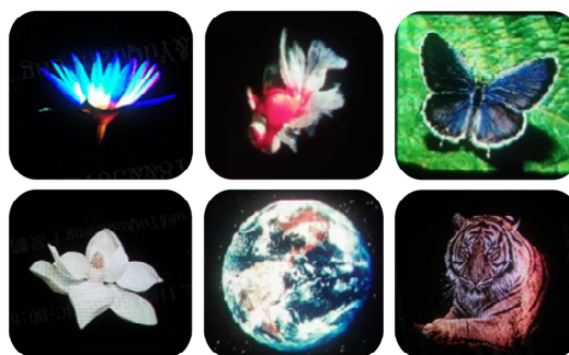
Fig. 6 Photos of the 1.1-inch 228-ppi QDCF micro-LED prototype, its specification, and display images.
