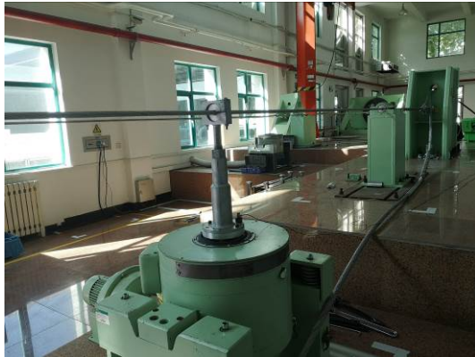
Fig. 5 Vibration exciter for simulating aeolian vibration.
