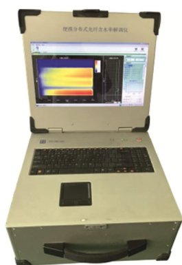
Fig. 27 Portable heating DTS moisture meter (developed by Suzhou Nanzhi Sensing Technology Co., Ltd.).
