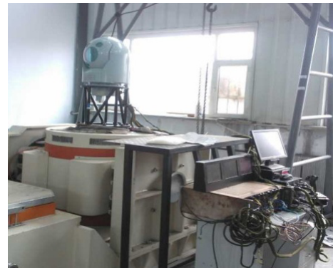
Fig. 2 Indoor test of the airborne PAT system.
