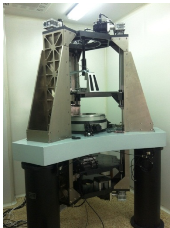
Fig. 8 Experimental lateral shearing interferometer.
