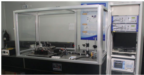
Fig. 1 Grating fabrication system of argon ion laser.
