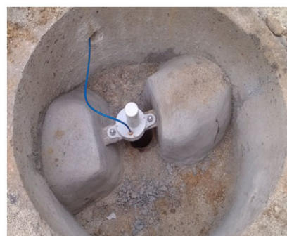
Fig. 7 Field installation of displacement sensor.
