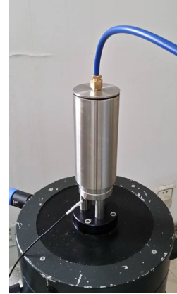
Fig. 3 Photograph of FBG-based micro-seismic sensor.
