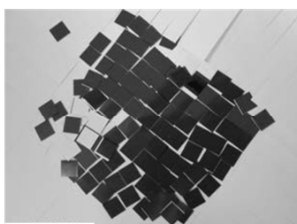
Fig. 2 Polyimide material as the sacrifice layer.
