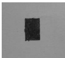
Fig. 4 ESL49000 material as the sacrifice layer.
