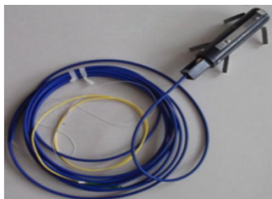
Fig. 6 Improved FBG geophone.
