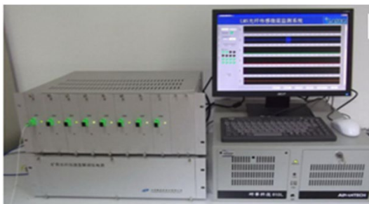
Fig. 7 Micro-seismic demodulator and data processor.
