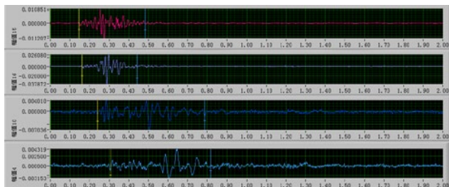
Fig. 8 Micro-seismic signals got by the FBG system.
