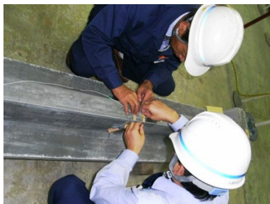
Fig. 6 Optical fiber sensor installation on the specimen.
