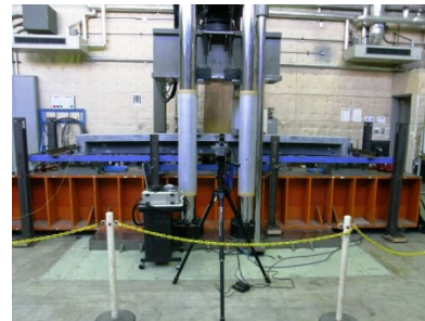
Fig. 7 Four-point bending experiment.
