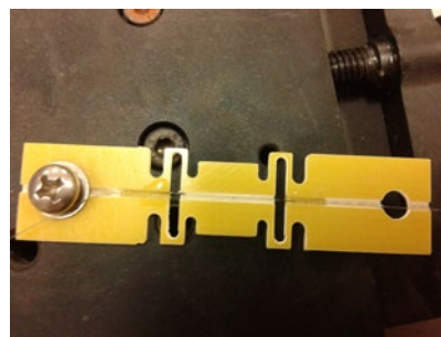
(b) FBG strain sensor packaged with FR-4
