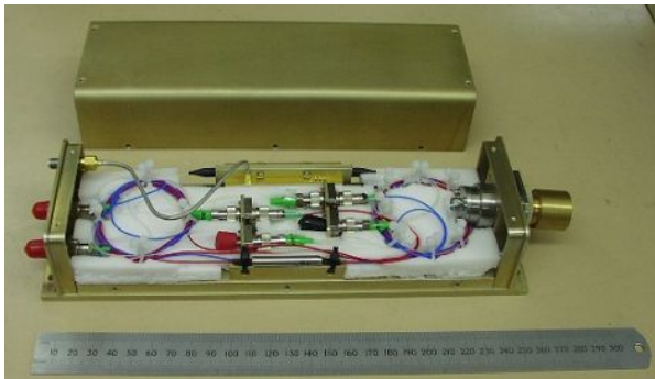
Fig. 20 SIPODs fiber Mach-Zehnder interferometer incorporating balanced phase modulators for carrier generation and symmetric circulators for output coupling.
