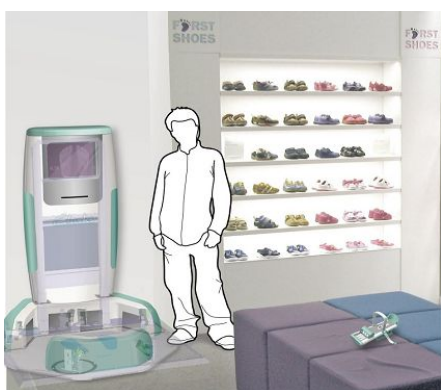
Fig. 18 Final shape measurement system as developed for Clarks provides six sets of 4800 range values (courtesy of Clarks).
