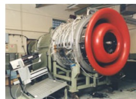
Fig. 14 4-stage axial research compressor at Cranfield with fiber optic laser anemometer mounted on left hand side.
