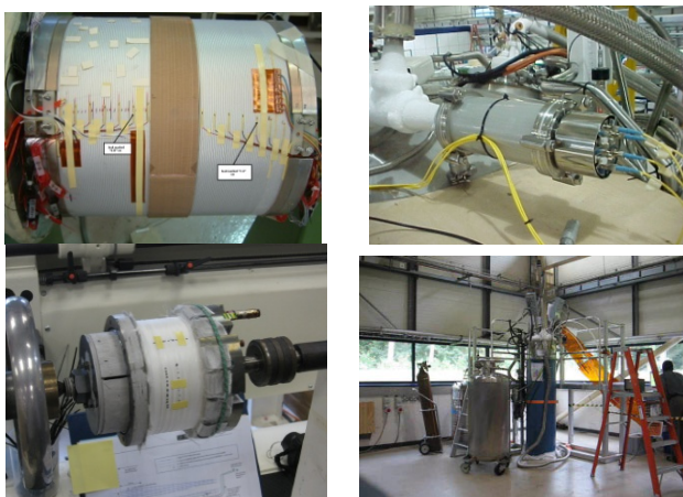
Fig. 45 FBG sensors deployed in superconducting magnets.
