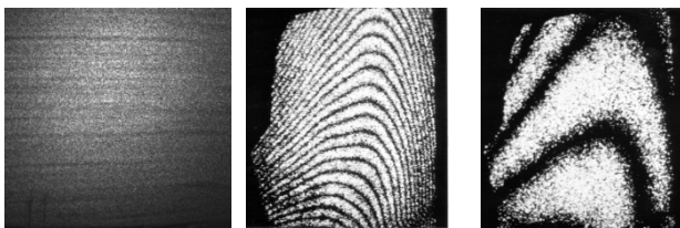
Fig. 19 Left–speckle image; middle and right–contour fringes of a gas turbine compressor blade: 190 GHz optical frequency modulation giving 0.9 mm fringes (middle) and 18.4 GHz optical frequency modulation giving 8 mm fringes (right).
