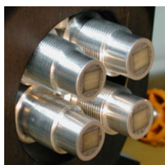
Fig. 11 Coherent imaging fiber bundles (600×500 fibers in each leg) in threaded mounts to enable couple to imaging systems.
