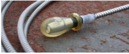
Fig. 20 Water-filled topcoat to prevent dehydration of the pH sensitive membrane (photo: STUMP GmbH).
