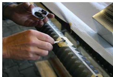
Fig. 8 Application of FBG sensor to the steel bar.
