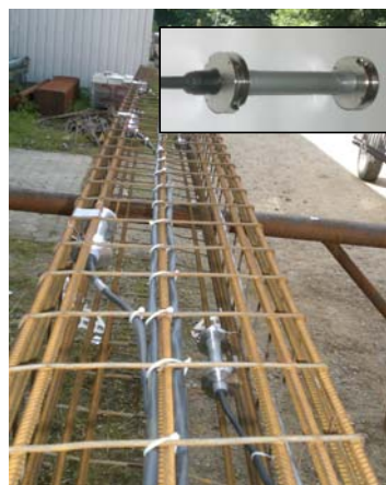
Fig. 4 Sensors fixed at the cage of reinforcement for a 19-m-length concrete pile (above right: sensor body).
