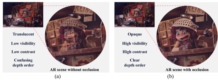
Fig. 1. Simulated AR scene (a) without occlusion and (b) with occlusion by Blender. In the pictures, the merchant and store are regarded as a virtual image and a real scene, respectively. The transparency of the merchant in (a) and (b) was set to 50% and 0%, respectively, to simulate the conventional and occlusion-supported AR scene. Source image: “The Junk Shop” by Alex Treviño. Original concept by Anaïs Maamar.
