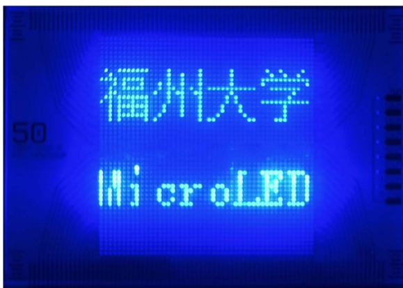
Fig. 3. Images of the 50 \mu\text{m} micro-LED array ( 48 \times 48 ) in operation. Both Chinese characters and English characters are shown in the display.
