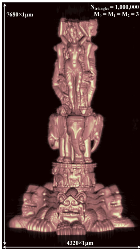
Fig. 19. Numerical reconstruction of the ultra-high-resolution hologram of the Thai statue. The Thai statue contains 1,000,000 triangles and is subdivided by M_0 = M_1 = M_2 = 3 . The full running time in the pipeline is 607 s.
