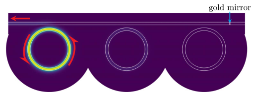
Fig. 7. Mode pattern |\psi| at the \text{EP}_6 for 3 microring cavities coupled to one WG with a gold mirror at the right side. Red arrows indicate the propagation direction of the field.
