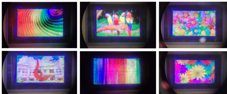
Fig. 7. The 4-bit full-color images demonstrated on the monolithically integrated full-color GaN-on-Si micro-LED microdisplay (demo videos see Visualization 1 and Visualization 2).
