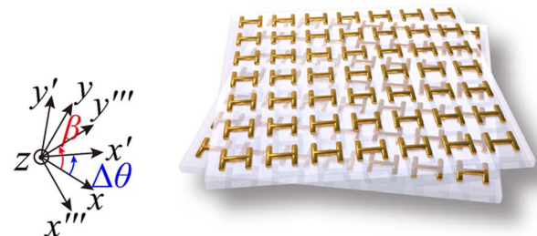
Fig. 9. Schematic diagram of the proposed moiré metasurface. Similar to Fig. 8, xyz and x'y'z are set as the coordinate systems of the bottom and top layers, respectively, while the x'''y'''z coordinates are used to describe the direction of the surface waves where the azimuthal angle \beta is defined as the one between the x and y''' directions.
