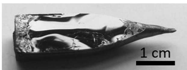
Fig. 6. Photograph of a p-InSe ingot cleaved parallel to the c -plane.
