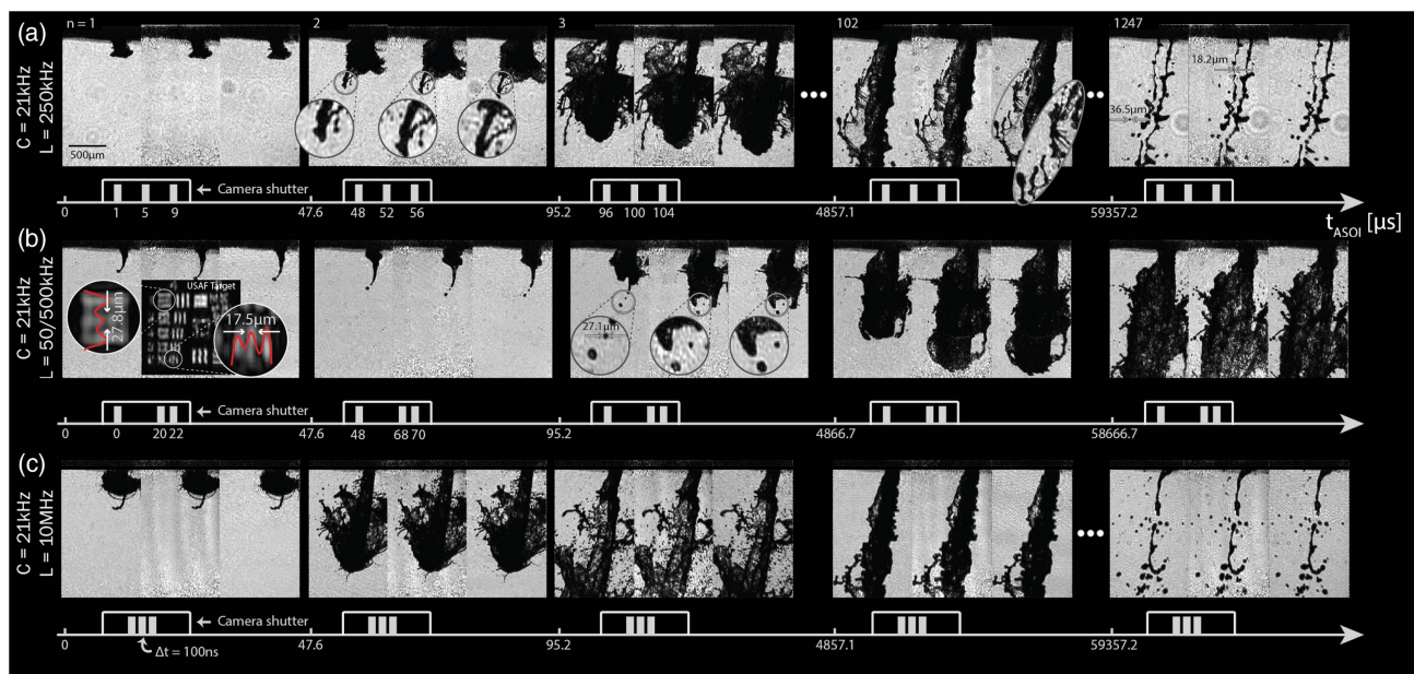
Fig. 2. Microscopic imaging of transient fluid dynamics at high speed. (a) Imaging the spray injection event at a camera speed of 21 kHz and a shutter time of 12 \mu s within which three pulses, with constant inter-pulse time (250 kHz FRAME triplet), are recorded. (b) Non-linear temporal triggering where the first two pulses arrive at the sample with an inter-pulse time of 20 \mu s (50 kHz), while the last two are incident with an inter-pulse time of 2 \mu s (500 kHz). At the beginning of the event, 50 kHz suffices to track the fluid's evolution within the camera exposure, while already at 95 \mu s ASOI, higher speeds are necessary. The zoom-ins of the USAF 1951 resolution target correspond to the resolution limits in x and y of the current optical configuration. (c) Imaging the injection event with 21 kHz camera speed and 10 MHz FRAME triplet (100 ns inter-pulse time) while retaining the image spatial resolution of (b). See Visualization 1 , Visualization 2 , Visualization 5 , and Visualization 6 for videos of the entire events.
