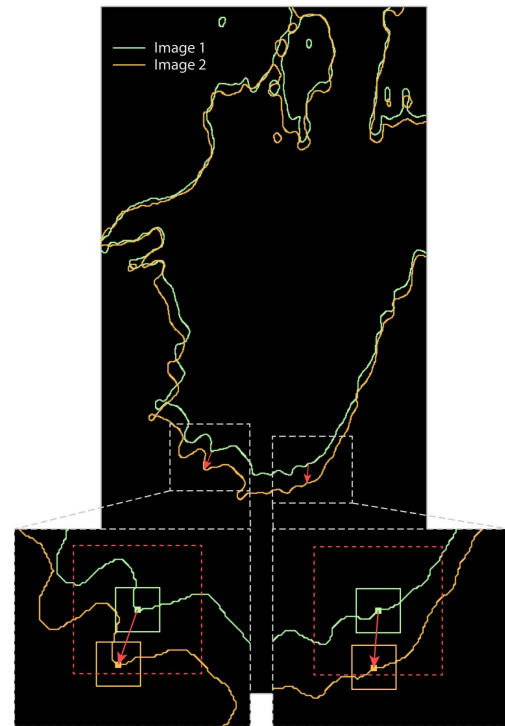
Fig. 7. Extraction of velocity vectors for each pixel along the segmentation edge. Two examples of where the initial template (green boxes) is scanned within a search area (red dashed boxes) across the subsequent image (outlined in orange). The template is placed at the position of maximum cross-correlation (orange boxes). The velocity vector is then calculated as the distance between the two center points divided by the inter-image time. This process is performed for every pixel along the segmentation edge.
