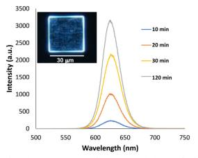
**Fig. 16.** Fluorescence intensity from QDs attached on 2D flat functionalized polymer structure (see inset) with respect to the immersion time (min). The excitation laser is at 405 nm with a power of 2  $\mu$ m, and the collection time is kept at 0.1 s. The left top small image (inset) is the dark-field image of the 2D flat polymer square.
