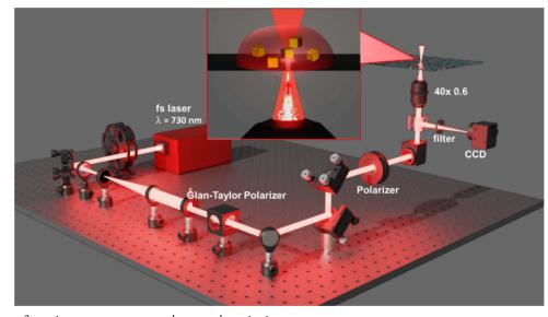
Fig. 7. Optical configuration to carry out two-photon polymerization.
