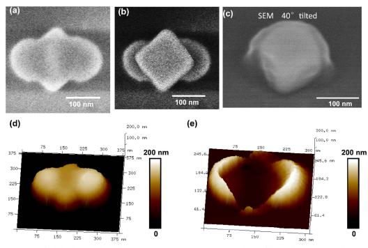
**Fig. 12.** (a) SEM image of a hybrid nanocube without attaching any QDs/polystyrene spheres (fabricated using 50% Dth). (b) Mixed image, the original SEM image of the cube before exposure is superimposed to (a). (c) 40-degree tilted SEM image. (d) 3D height image measured by AFM of the same hybrid nanocube as (a). (d) 3D height image subtracted by the original cube's height profile from (c), demonstrating the 3D polymer distribution.
