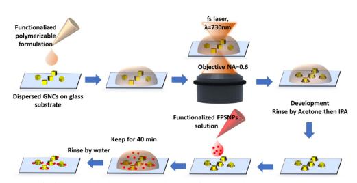
Fig. 6. The process steps for fabricating hybrid FPS-attached cubes (FPS: fluorescent polystyrene sphere).
