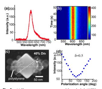
**Fig. 3.** (a) Fluorescence spectrum measured from the hybrid FPSs–GNC shown in Fig. 2(a) using polarized green laser of 532 nm wavelength for excitation. A 650/150 nm bandpass filter is used to separate the fluorescent signal from the incident excitation. (b) Spectrum time trace, collected for 50s. (c) Definition of the polarization angle for excitation. (d) Fluorescence intensity as a function of the angle of incident polarization defined in (c).
