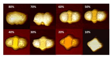
Fig. 10. AFM images of some hybrid GNCs with attached QDs, fabricated using incident doses from 80% decreasing to 10% of Dth (Step 1).
