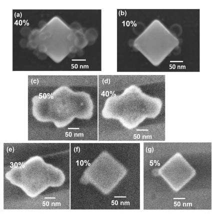
**Fig. 9.** More examples of hybrid FPS-attached GNCs. (a), (b) SEM images of the hybrid FPS-attached nanocubes fabricated using 40% Dth and 10% Dth, and the residence time of the FPS solution is 40 min. A 10 kV voltage is used for SEM observation. (c)–(g) FPS-attached nanocubes fabricated separately using 50% Dth, 40% Dth, 30% Dth, 10% Dth, and 5% Dth. The immersion time of the sample in the FPS solution is decreased to 10 min. A 1 kV voltage is used for SEM observation.
