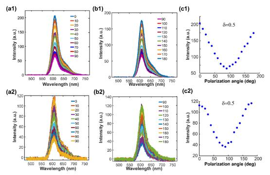
**Fig. 11.** Emission spectra from two hybrid FPS-attached GNCs fabricated using same parameters, and their exposure dose is 40% Dth. (a1) and (b1) The emission spectra from the first hybrid FPS-attached GNC when the polarization angle of the laser used for the excitation varies separately from 0 deg to 90 deg and 90 deg to 180 deg. (c1) The emission peak intensity changing trend. (a2), (b2), and (c2) The results from the second hybrid FPS-attached GNC.
