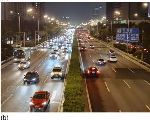
**Fig. 10.** Photos of the traffic condition at the target vibration location. (a) The typical traffic picture before 23:00. Vehicles on the road are mainly light-weight cars, which will cause low-amplitude high-frequency fluctuations. (b) The typical traffic picture after 24:00. Cargo lorries are permitted to enter the downtown city, which will produce high-amplitude low-frequency shockwaves.
