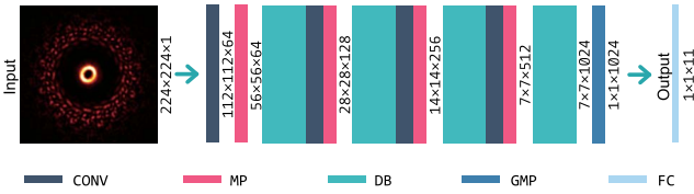
Fig. 2. Schematic diagram of DenseNet-121. CONV, convolution layer; MP, max pooling layer; DB, dense block; GMP, global max pooling layer; FC, fully connected layer.
