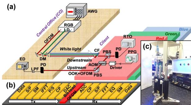
**Fig. 1.** (a) Experimental setup of tricolor RGB LD-based bidirectional VLC system. (b) OFDM signal encoding and decoding processes. (c) Photography of tricolor RGB LD to produce white light. AWG, arbitrary waveform generator; PBS, polarization beamsplitter; DM, dichroic mirror; PD, photodiode; RTO, real-time oscilloscope; CF, color filter; AOM, acousto-optic modulator; ED, error detector; PPG, pulse-pattern generator; LPF, low pass filter.
