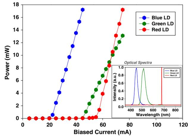
**Fig. 2.** Experimental output optical power and biased current responses of the RGB LDs. Inset: measured optical spectra.
