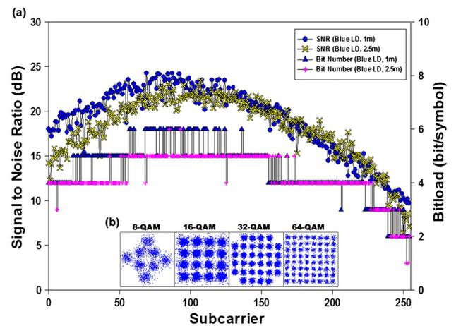
**Fig. 5.** (a) Measured SNRs and bit-loading of different OFDM subcarriers. (b) Constellation diagrams of 8, 16, 32, 64-QAM of blue LD.
