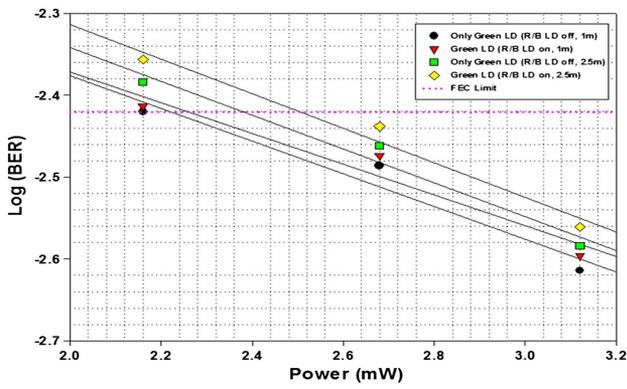
**Fig. 7.** Measured log(BER) of green LD at different received powers and influence on green LD with R/B LDs off and R/B LDs on.
