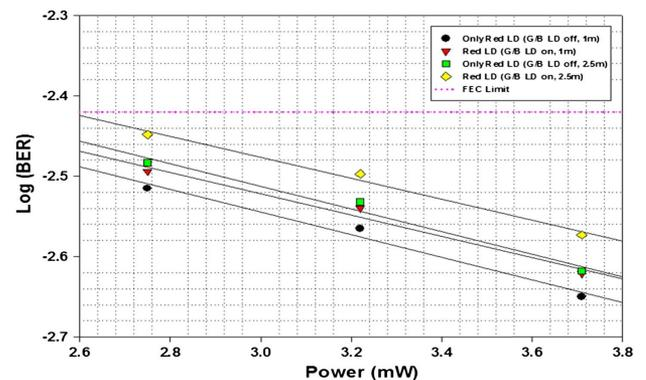
**Fig. 6.** Measured log(BER) of red LD at different received powers and influence on red LD with G/B LDs off and G/B LDs on.
