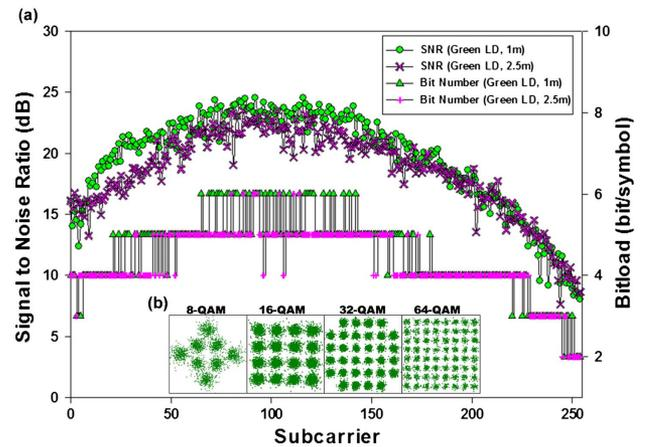
**Fig. 4.** (a) Measured SNRs and bit-loading of different OFDM subcarriers. (b) Constellation diagrams of 8, 16, 32, 64-QAM of green LD.
