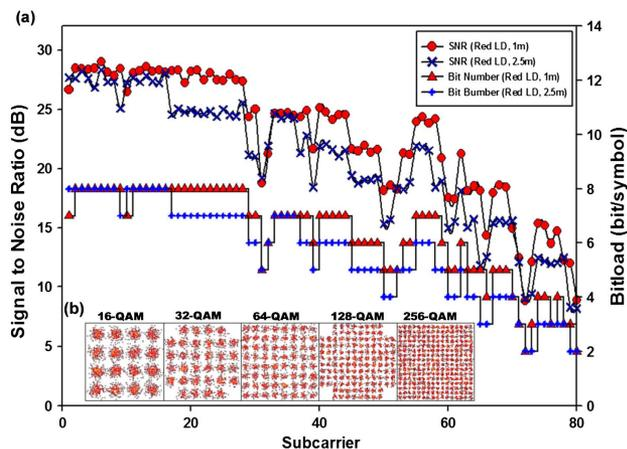
**Fig. 3.** (a) Measured SNRs and bit-loading of different OFDM subcarriers. (b) Constellation diagrams of 16, 32, 64, 128, 256-QAM of red LD.
