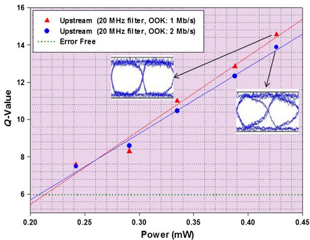
**Fig. 9.** Measured  $Q$ -value of the remodulated upstream OOK signal (red points: 1 Mbit/s, blue points: 2 Mbit/s) against different received optical powers when different LPFs are used.
