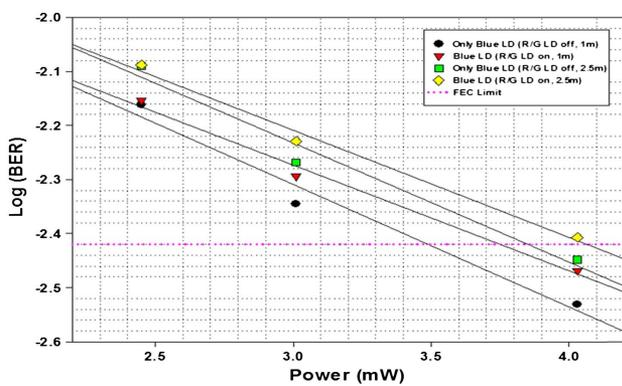
**Fig. 8.** Measured log(BER) of blue LD at different received powers and influence on blue LD with R/G LDs off and R/G LDs on.
