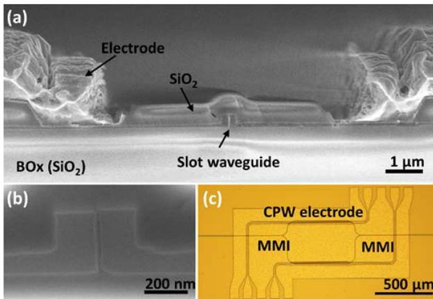
**Fig. 3.** (a) Cross-sectional SEM image of the fabricated modulator across the active region. (b) Magnified view of the MOS capacitor at the rib section, where the oxide layer is clearly visible. (c) Optical image of the fabricated MZI modulator with 500- $\mu\text{m}$ -long phase shifter.
