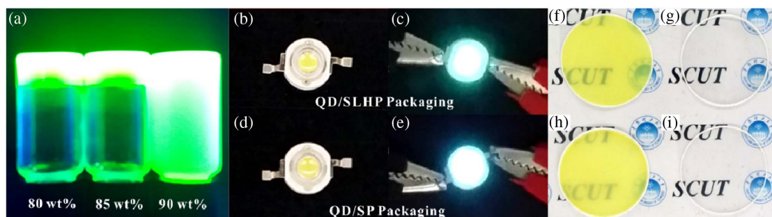
Fig. 1. (a) SLHP with methyl-PDMS concentrations of 80 wt. %, 85 wt. %, and 90 wt. % after curing at 125°C for 90 min, respectively. (b)–(c) LED images with QD/SLHP packaging structure (concentrations of QDs and methyl-PDMS are 0.8 and 85 wt. %, respectively) under injection currents of 0 and 2 mA, respectively. (d)–(e) LED images with QD/SP packaging structure (concentrations of QDs and methyl-PDMS are 0.8 and 0, respectively) under injection currents of 0 and 2 mA, respectively. Images of (f) QD/SP film (0.3 wt. % QDs), (g) SP film, (h) QD/SLHP film (0.3 wt. % QD and 85 wt. % methyl-PDMS), and (i) SLHP film (85 wt. % methyl-PDMS).
