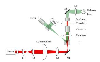
**Fig. 1.** Experimental schematic diagram of the LOT setup. L1, lens 1; L2, lens 2; L3, lens 3; M1, reflection mirror 1; D1, dichroic mirror; M2, reflection mirror 2; L4, lens 4.
