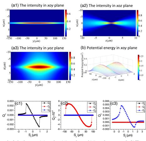
**Fig. 2.** Electric field amplitude distributions in (a1) *xoy* plane, (a2) *xoz* plane, and (a3) *yoz* plane, respectively. (b) The trapping potential energy surface calculated for the line optical trap in *xoy* plane. The optical trapping efficiencies (c1)  $Q_x \sim S_x$ , (c2)  $Q_y \sim S_y$ , and (c3)  $Q_z \sim S_z$  on a PS particle imposed by the LOT.
