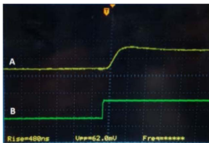
Fig. 4. Detected signal from the photodetector (signal A) and modulation signal of the MMW/THz radiation (signal B). The response time of the detection using the PDB210A photodetector was found to be 480 ns.
