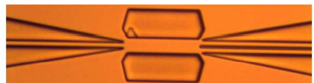
Fig. 4. Low reflection splitters: photograph of a 1 \times 2 MMI splitter [22].
