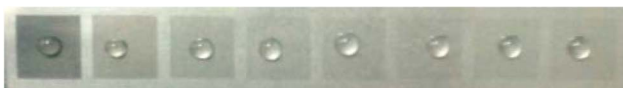
Fig. 1. Image of the treated areas under different parameters. From the first to the eighth areas, scanning speeds and intervals are 400 \mu\text{m/s} and 20 \mu\text{m} , 1000 \mu\text{m/s} and 40 \mu\text{m} , 2000 \mu\text{m/s} and 60 \mu\text{m} , 3000 \mu\text{m/s} and 80 \mu\text{m} , 4000 \mu\text{m/s} and 100 \mu\text{m} , 5000 \mu\text{m/s} and 120 \mu\text{m} , 6000 \mu\text{m/s} and 140 \mu\text{m} , 7000 \mu\text{m/s} and 160 \mu\text{m} , respectively.
