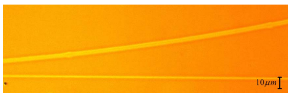
Fig. 5. Top-view microscope image of parts of bus and ring waveguides, directly written in a thin layer of \text{As}_2\text{S}_3 .
