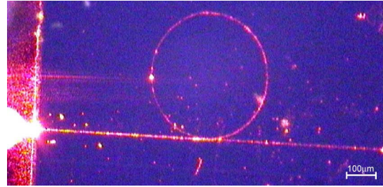
Fig. 6. Top view of a ring resonator waveguide, directly written in an \text{As}_2\text{S}_3 thin film. Red light is coupled from a tapered fiber for illustration purposes only.
