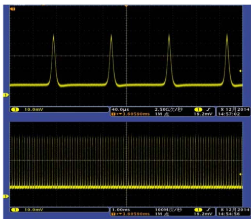
Fig. 2. Q-switching pulse train in 400 μs and 10 ms timescales, respectively.
