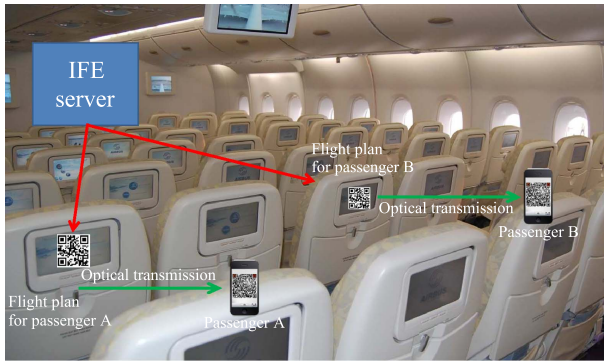
Fig. 2. Setup for the transmission of passenger-specific data.
