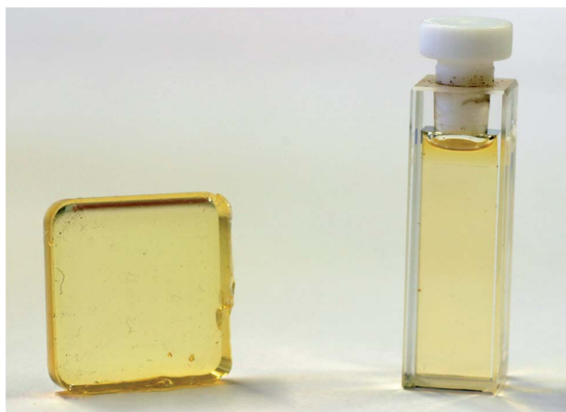
Fig. 1. Solid-state sample of OSO embedded in PDMS (left) and the commonly studied solution of OSO in DCM in a cuvette (right).
