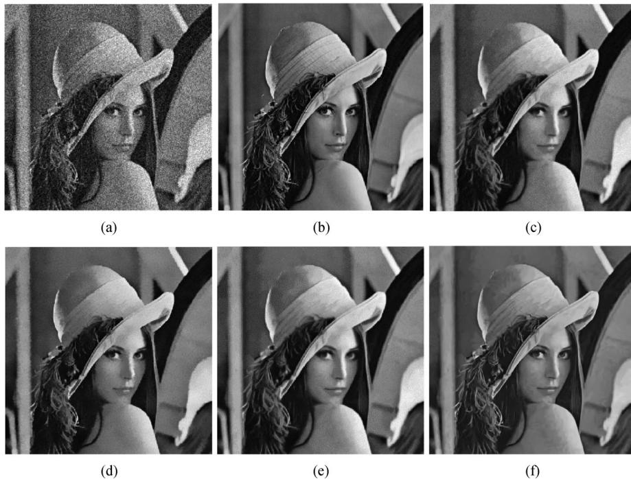
Fig. 4 Lena images. (a) Noise image; (b) standard image; (c) denoised by WNNM; (d) denoised by NLM; (e) denoised by NLM-WNNM; (f) denoised by BM3D
