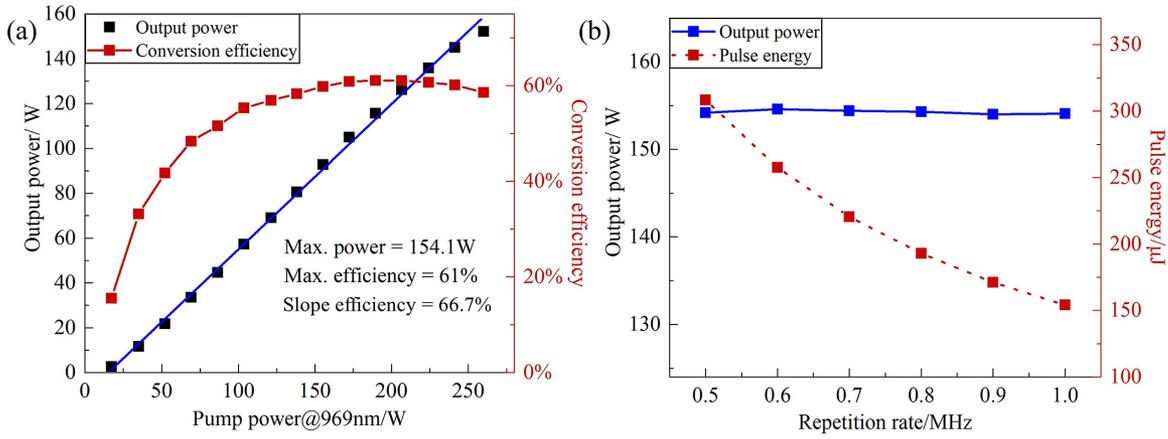
**Figure 5.** Power characteristics of the thin-disk regenerative amplifier. (a) Pump power versus output power and efficiency at 1 MHz. (b) Average power and pulse energy at the maximum power repetition rate.
