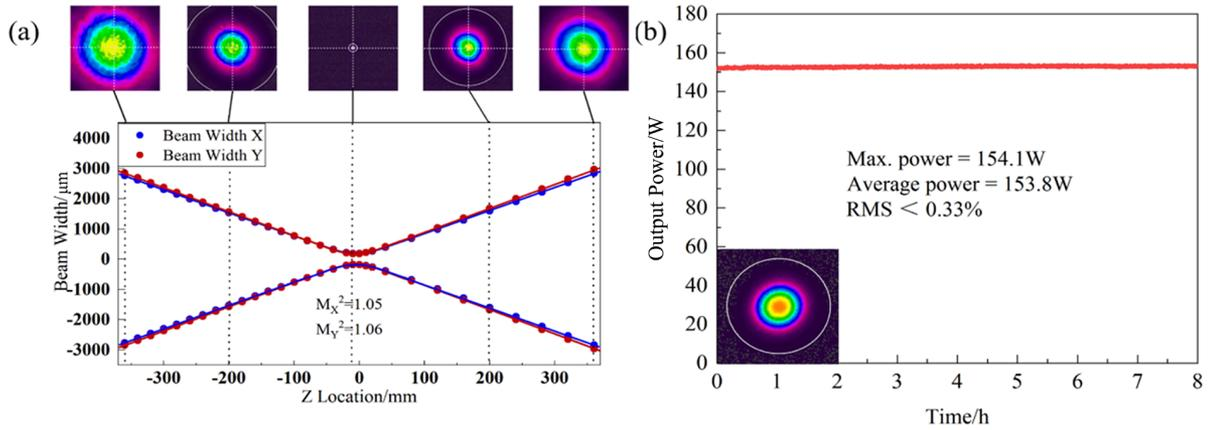
**Figure 8.** (a) Beam quality of the laser at 154.1 W. (b) Power stability of the laser at 154.1 W.
