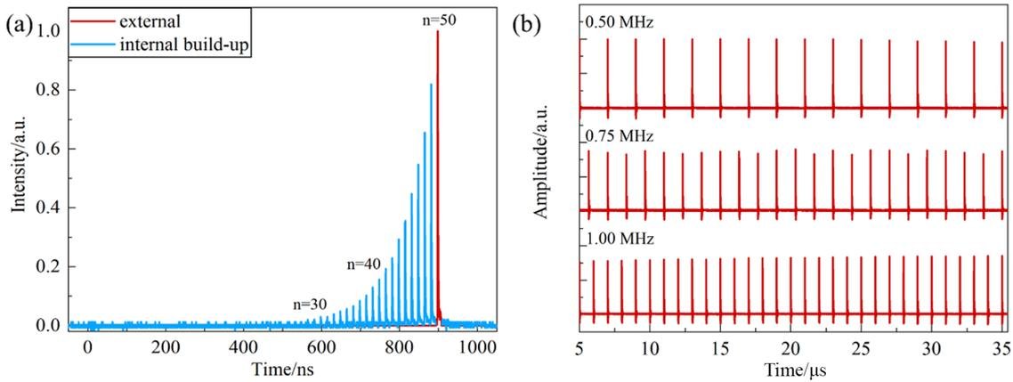
**Figure 6.** Temporal characteristics of the thin-disk regenerative amplifier. (a) Intracavity pulse build-up;  $n$ , number of roundtrips. (b) Temporal pulse trains.
