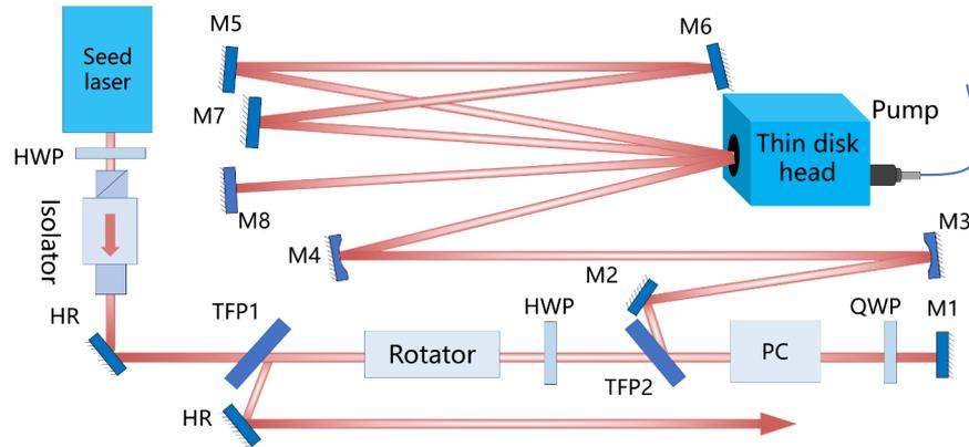
**Figure 1.** Optical scheme of the regenerative amplifier. HWP, half-wave plate; QWP, quarter-wave plate; TFP1, TFP2, thin film polarizer; PC, Pockels cell; M1, M2, M5–M8, mirror; M3, M4, concave mirror.
