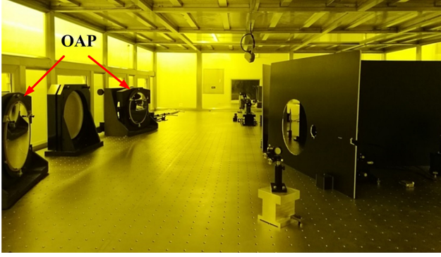
Figure 2. Reflective two-beam laser static interference lithography station for MLD grating fabrication.
