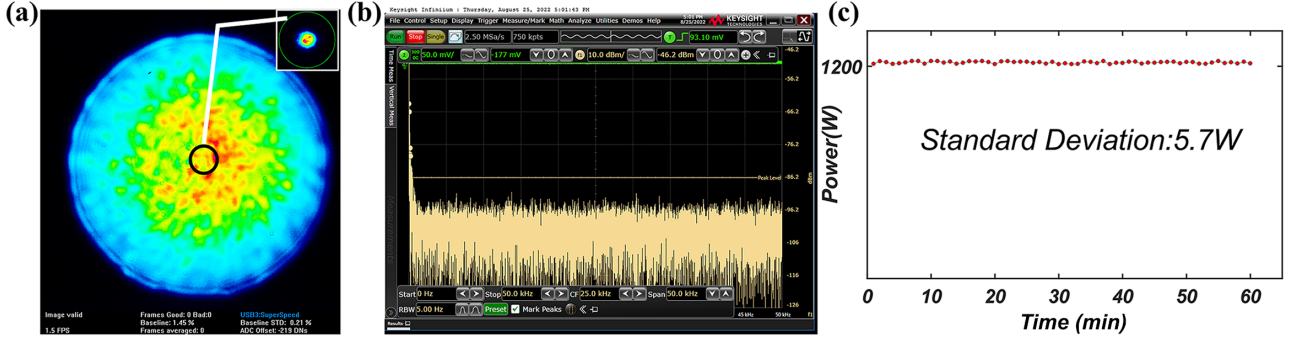
Figure 5. Output stability of the system. (a) With a full collimated beam captured by a charge-coupled device (CCD); (inset) sampling spot selected by pinhole; (b) Fourier transform of the temporal trace; (c) power stability within 1 hour.
