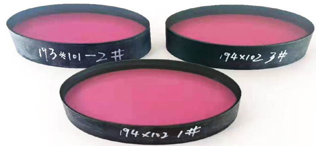
Figure 9. Monolithic edge-cladding N31 elliptical disks with the size of 200 mm × 108 mm × 40 mm. The thickness of the cladding layer can be about 2–20 mm as designed.
