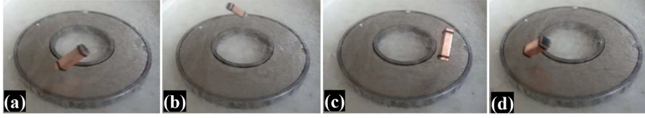
Figure 13. Quantum locking based on the flux pinning effect makes the HTSC-sabot orientation fixed in space so that it will not re-orient itself without any external action (the HTSC-sabot temperature is \sim 80 K).
