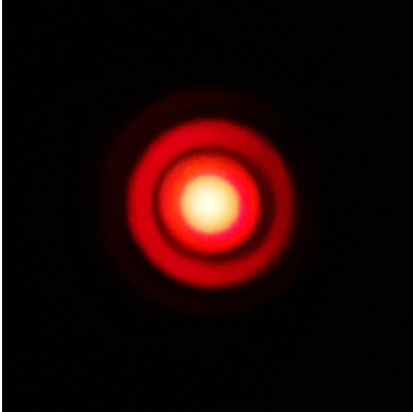
Figure 4. The beam profile of the compressed pulses after the two-stage configuration, just before final compression. The profile is collected by imaging a flat piece of paper in the beam, imaged onto a camera.
