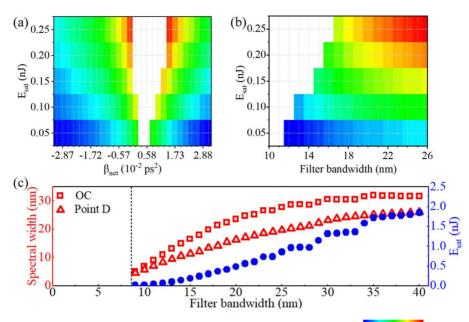
**Figure 6.** (a) FWHM spectral width of output pulses as a function of NCD and  $E_{sat}$ . Linear scale: 4 nm 20 nm (white area: multi-pulsing region). (b) FWHM spectral width of pulses at point D as a function of filter bandwidth and  $E_{sat}$ . Linear scale: 8 nm 20 mm (white area: multi-pulsing region). (c) FWHM spectral width of pulses at the OC (red open squares) and at point D (red open-triangles) at critical pump power and corresponding  $E_{sat}$  (blue solid circles).
