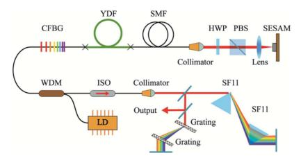
Figure 1. Experimental setup of the passively mode-locked all-PM fiber laser. LD, laser diode; WDM, wavelength division multiplexer; CFBG, chirped fiber Bragg grating; YDF, Yb-doped fiber; SMF, single-mode fiber; SESAM, semiconductor saturable absorber mirror; HWP, half-wave plate; PBS, polarization beam splitter; ISO, isolator.
