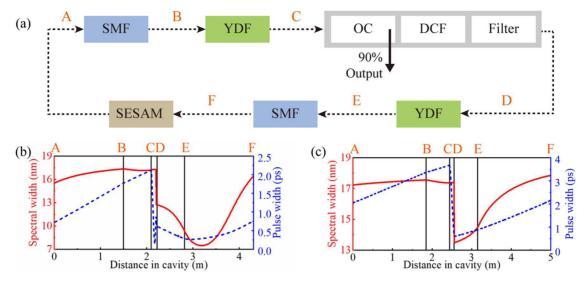
**Figure 5.** (a) Schematic of the numerical simulation model. Evolution of spectral width (red solid line) and temporal width (blue dotted line) when the NCD is for (b)  $\beta_{\text{net}} = -1.1 \times 10^{-3} \text{ ps}^2$  and (c)  $\beta_{\text{net}} = +1.5 \times 10^{-2} \text{ ps}^2$ . YDF, Yb-doped fiber; SMF, single-mode fiber; SESAM, semiconductor saturable absorber mirror; DCF, dispersion compensating fiber; OC, optical coupler.
